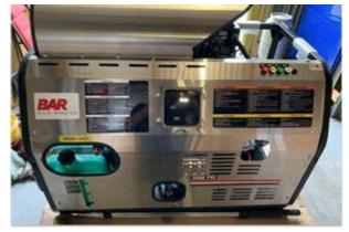
**Frame:** Powder coated steel square tube skid frame · Stainless-steel removable front panel · Optional wheel kit with locking tire brake, four tires and solid steel threaded axles
