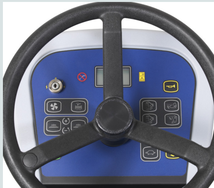
Control panel with icon buttons and modern display to reach best in class ease of use
