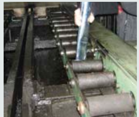
Vacuuming grinding sludge
